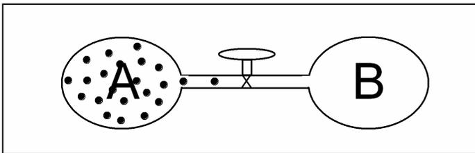
Fig. 1. The classical demonstration of entropy change described by the Second Law of Thermodynamics. An increase in entropy is produced when the gas in chamber A is allowed to pass through the valve into the vacuum of chamber B.
